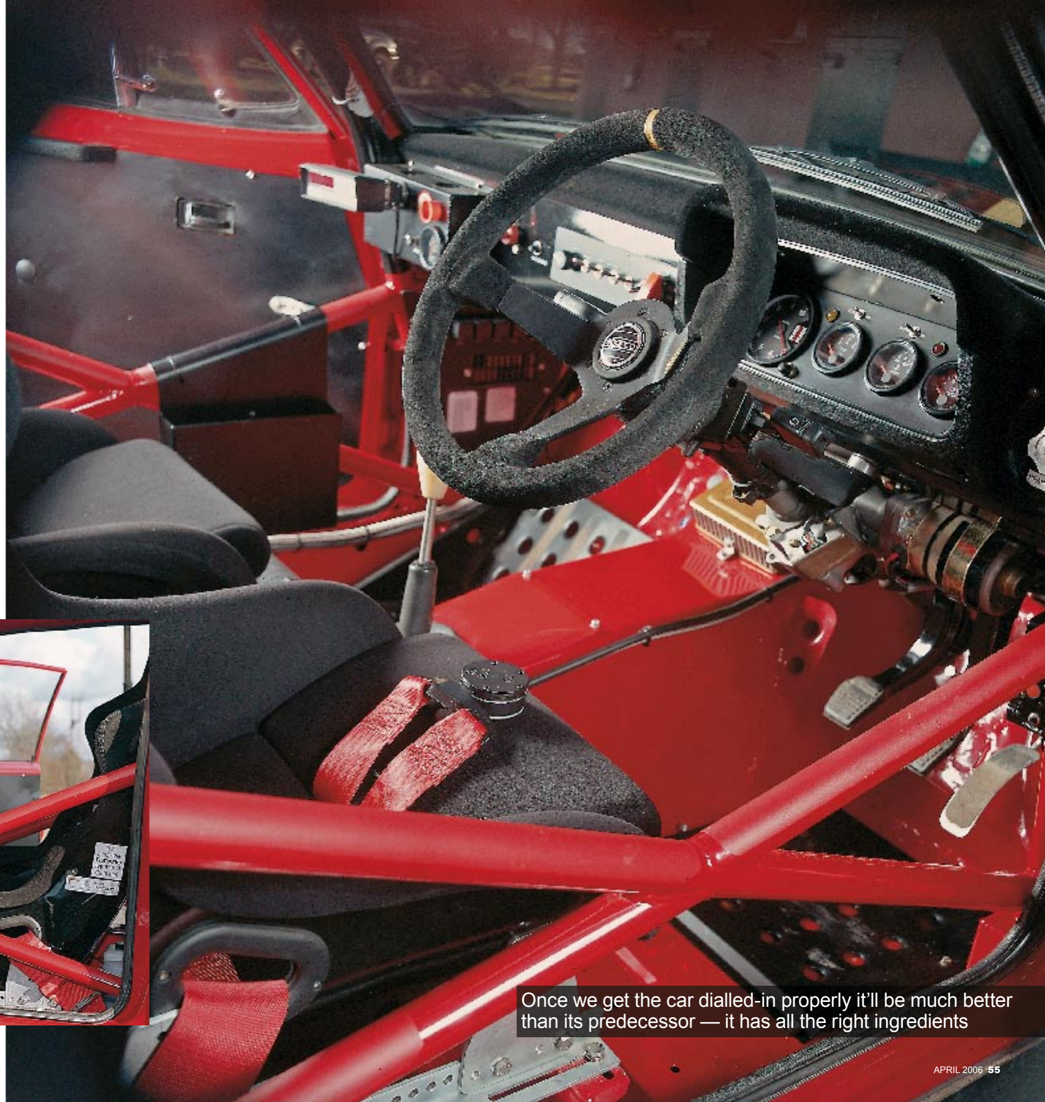
This is proper rally kit! Light, powerful and as stiff as they come. Between the 2.4 Holbay/Warrior is 300 brake horse and some of the trickiest suspension available. Jason's car will be a real force to be reckoned with on the stages.
